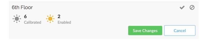
The panel shows the count of calibrated and enabled nodes in the area. If there are no calibrated nodes, a corresponding message (similar to on area selection) is shown instead:
